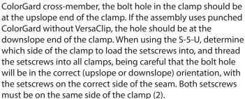
3. Installing the clamps: S-5! clamps are installed differently depending upon clamp model and seam style. Please see the installation instructions included with your clamps. For maximum holding strength, setscrews should be tensioned and re-tensioned as the seam material compresses. Screw tension should be verified using a calibrated torque wrench between 160 and 180 inch pounds when used on 22ga steel and between 130 and 150 inch pounds for all other metals and
