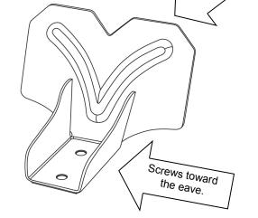
Failure to install an adequate amount of snow guards and in the proper pattern will void the warranty.
